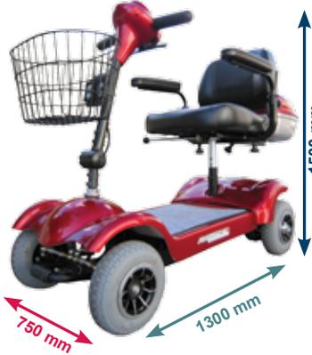
A side-view diagram of a red mobility scooter with a black seat and a wire basket. Dimension lines indicate a width of 750 mm, a length of 1300 mm, and a height of 1500 mm.
